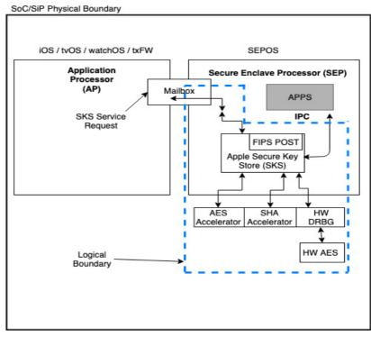
Figure 1: Cryptographic Module Block Diagram
